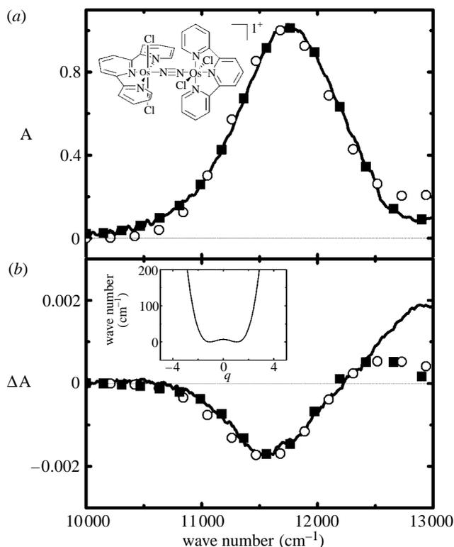
Figure 6. (a) Absorption and (b) Stark spectra of **6** in 1 : 1 propionitrile/butyronitrile at 77 K. Data (solid lines) fit to the classical model (filled squares) and the non-classical model (open circles) are shown, along with the groundstate potential energy surfaces derived from the non-classical model (inset). Fit parameters are listed in table 1.
