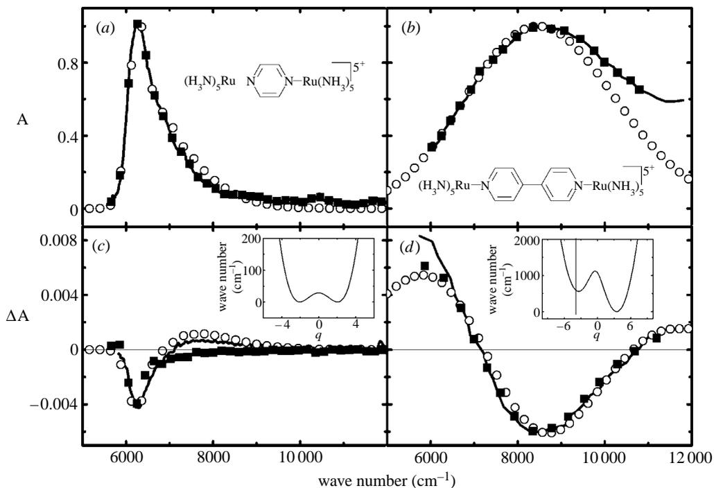
Figure 4. (a,b) Absorption and (c,d) Stark spectra of **1** and **2** in 1 : 1 water/glycerol at 77 K; counter ions are  $(\text{C}_7\text{H}_7\text{SO}_3^-)_5$  and  $(\text{Br}^-)_5$ , respectively. Data (solid lines) fit to the classical model (filled squares) and the non-classical model (open circles) are shown, along with the groundstate potential surfaces derived from the non-classical model (inset). Fit parameters are listed in [table 1](#).
