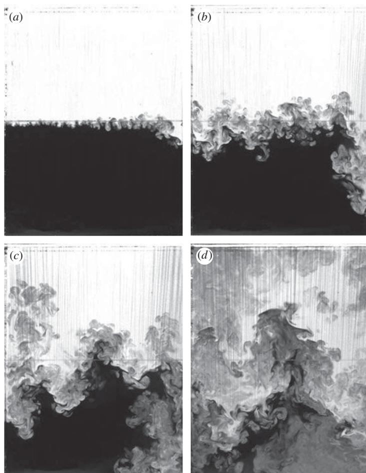
Figure 8. PLIF images of R–T evolution in a composite sliding plate experiment with  $A_t = 2 \times 10^{-3}$ . Times: (a)  $t=0$ , the end of barrier removal, (b)  $t=5$  s, (c)  $t=10$  s and (d)  $t=15$  s.
