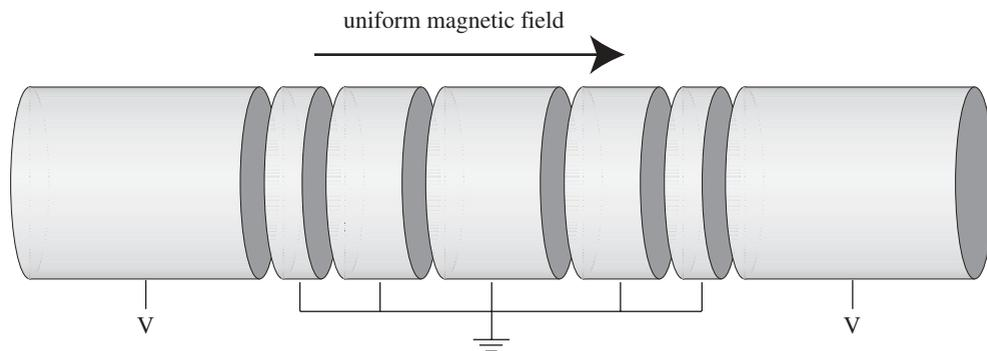
Figure 1. Example of a Penning–Malmberg trap similar to those used in the antihydrogen experiments. Particles are confined radially by a strong uniform axial magnetic field. Axially they are confined by the electric fields generated by biasing the conducting, but individually insulated, cylinders (called electrodes). In practice, more electrodes are needed for antiparticle manipulations and the ALPHA, ATHENA and ATRAP experiments use up to 50 individually controllable electrodes.
