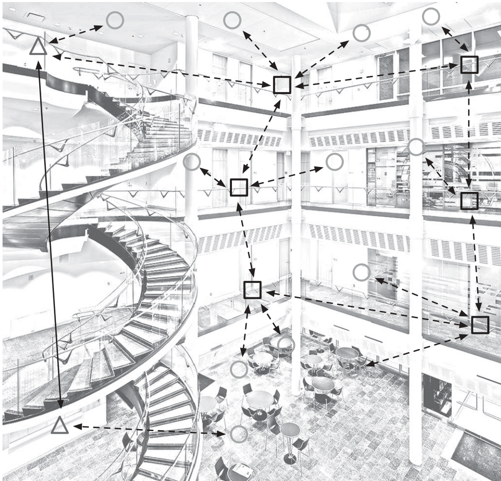
Figure 2. Sensor network elements and organization. Root nodes (triangles) connect the sensor network to external networks. Mesh nodes (squares) originate their own sensor and other data and forward traffic on behalf of other nodes. Leaf nodes (circles) are like mesh nodes, but they do not typically forward flow-through traffic.
