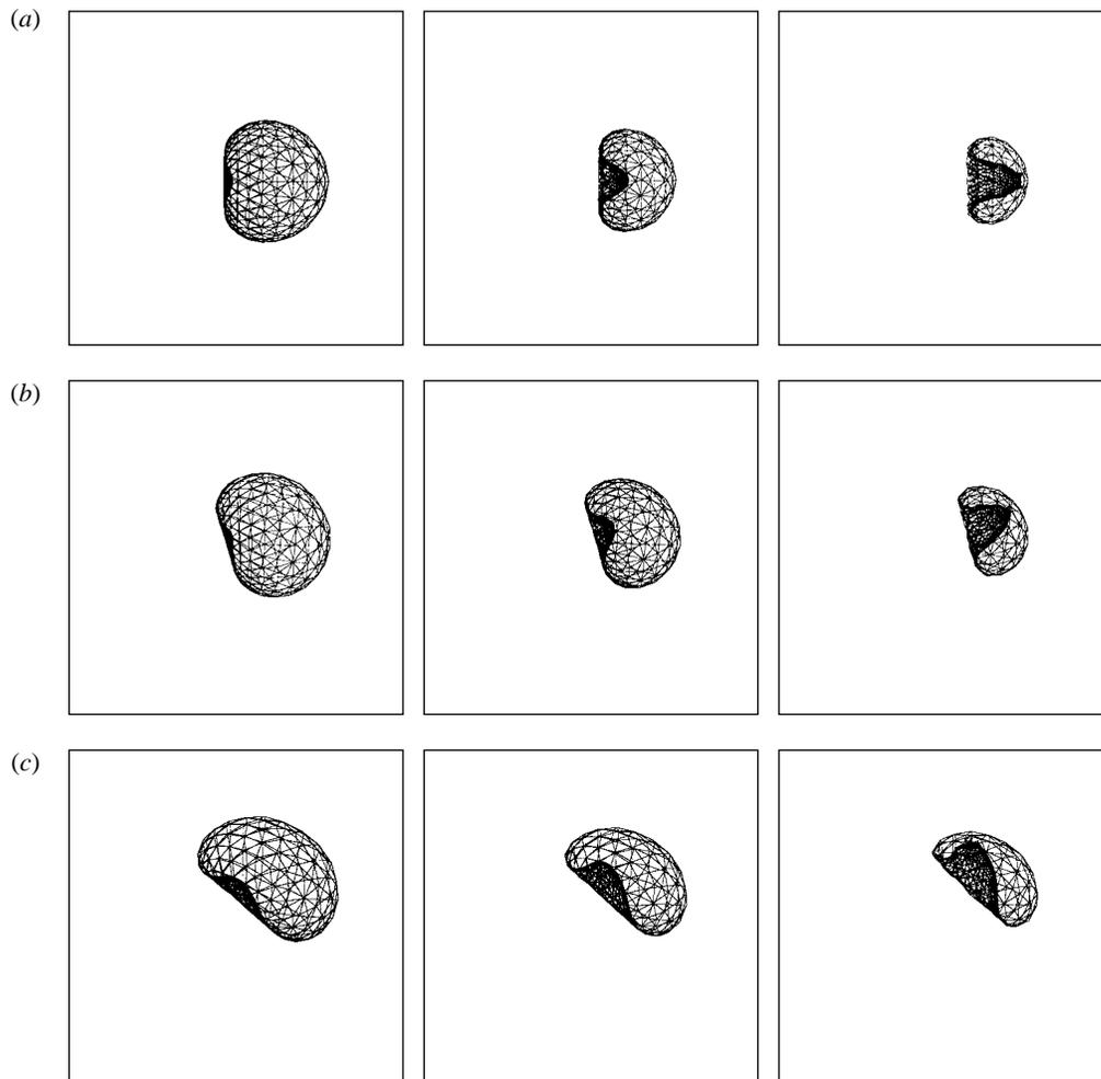
Figure 5. The expansion and collapse of an explosion bubble near a vertical wall for  $\gamma = 2.0$ , showing the effect of increasing the buoyancy parameter  $\delta$ : (a)  $\delta = 0$ ; (b)  $\delta = 0.1$ ; (c)  $\delta = 0.2$ .
