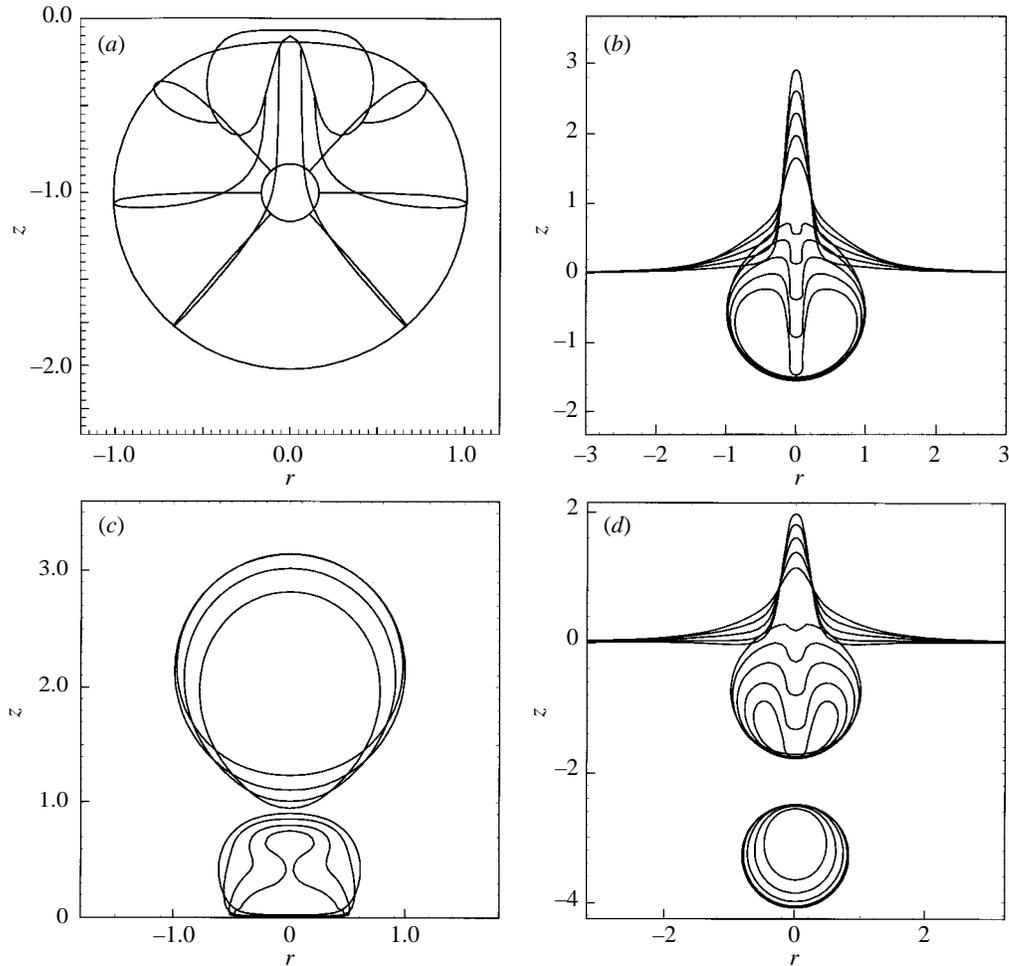
Figure 2. Vapour bubbles,  $\alpha = 0$ . (a) The particle paths during growth and collapse for a bubble below a rigid boundary,  $\gamma = 1.0$ ,  $\delta = 0$ . (b) The collapse of a single bubble near a free surface. (c) The collapse of two different sized bubbles above a rigid boundary. (d) The collapse of two bubbles beneath a free surface.
