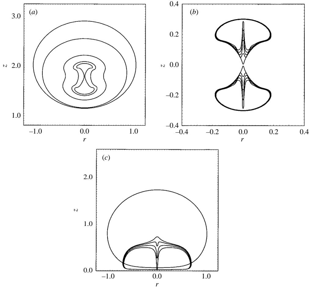
Figure 6. (a) Collapse of a vapour bubble in a stagnation point flow for  $\gamma = 2.31$ ,  $\beta = 0.126$ . (b) The ultra high speed jets that form during the collapse of a perturbed spherical bubble after it divides into two. (c) Collapse of a vapour bubble in a stagnation point flow for  $\gamma = 0.87$ ,  $\beta = 0.09$ .
