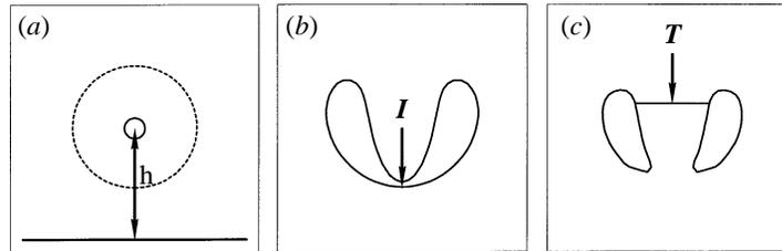
Figure 1. (a) The location of the point of bubble inception. (b) A cut is introduced at the point of impact,  $I$ , in order to continue to the toroidal phase. (c) An arbitrary cut,  $T$ , is introduced at each time step for the toroidal bubble.
