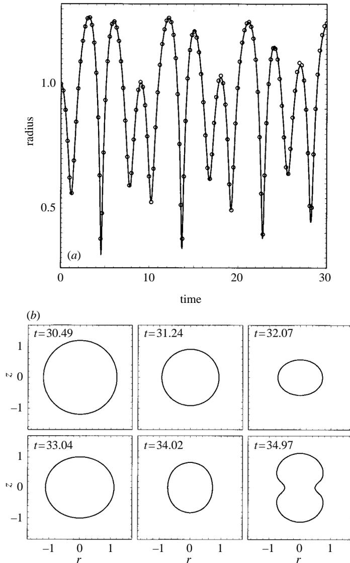
Figure 8. (a) Comparison between the radius-time curve calculated numerically by the boundary integral method (o) and the Rayleigh–Plesset equation (—). The corresponding parameters are given by  $\Omega = 524$  kHz,  $\Delta p = 1$  atm,  $p_a = 0.333$  atm,  $p_0 = 0.6$  atm and  $We = 35$ . (b) The bubble oscillations for  $t > 30$ , being the continuation of the boundary integral computation.
