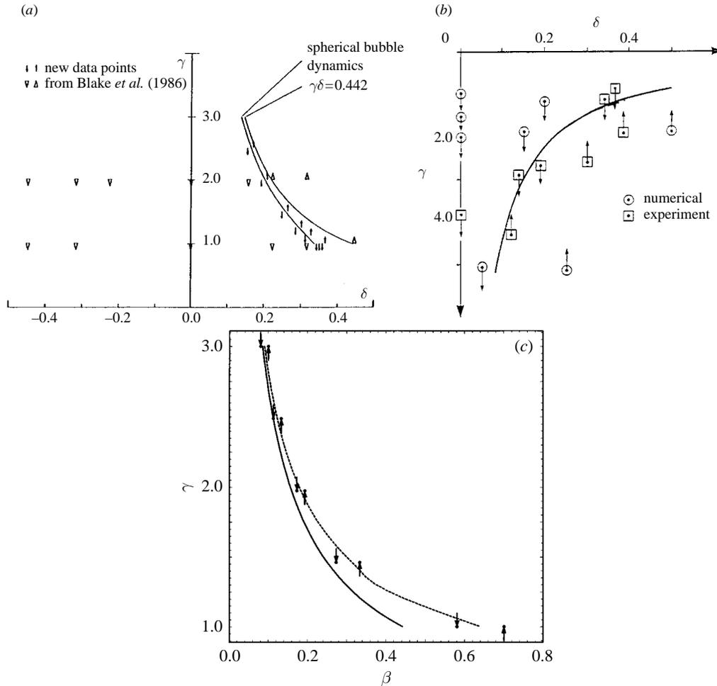
Figure 7. The null impulse curve for axisymmetric buoyant vapour bubbles ( $\alpha = 0$ ): (a) above a rigid plane boundary (the direction of the arrow or triangle denotes the direction of jet formation computed by the boundary integral method); (b) beneath a free surface; (c) in a stagnation point flow, (—) fixed spherical bubble, (---) translating spherical bubble.
