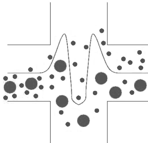
Figure 15. Filtering of particles of different sizes in the resonant regimes: larger particles stay in the lower part of the main channel, while smaller ones cross the interface; this is due to the fact that, in resonant regimes, the exchange area between the lower and upper parts of the flow is momentarily increased in the channel intersection.
