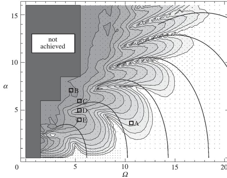
Figure 9. Contour plot of the folding quantity ( $F$ ) as a function of the control parameters ( $\Omega$ ,  $\alpha$ ): each measurement of  $F$ , points; states shown in figure 7, squares; and theoretical predicted resonances, solid lines.
