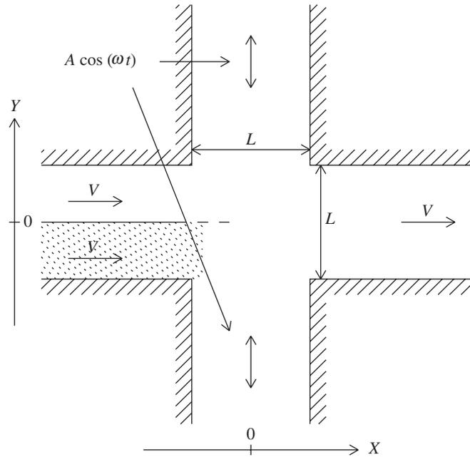
Figure 3. Schematic set-up of the active X-mixer with the characteristic quantities.
