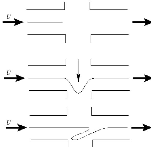
Figure 2. Stretching and folding of an incoming material line as it takes place in the X-mixer.
