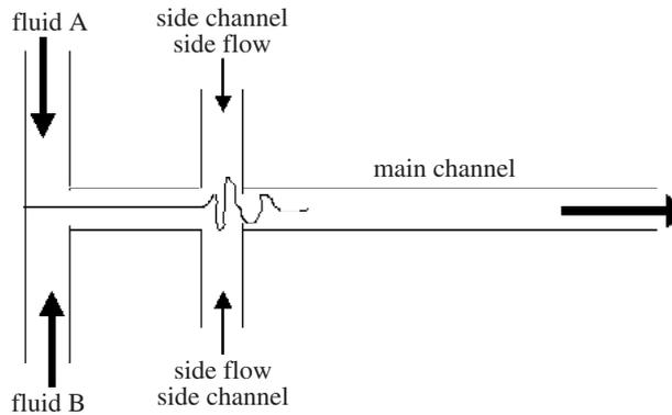
Figure 1. Sketch of the X-mixer. Two miscible fluids (A and B) are conveyed, side by side, towards a cross-channel intersection. At the intersection a time-dependent, additional side flow is driven favouring, under appropriate conditions, mixing between the two fluids.
