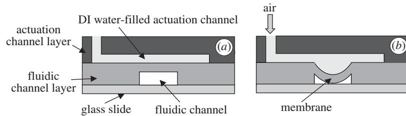
Figure 11. PDMS valve actuation: (a) working channel open; (b) working channel closed.
