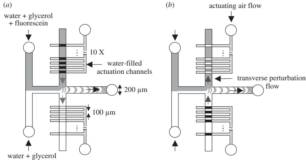
Figure 10. Layout of the experimental system used in the article with the operation mode: (a) upper valves closed, lower ones open, producing a side flow oriented downwards; (b) opposite movement, producing an upwards side flow.
