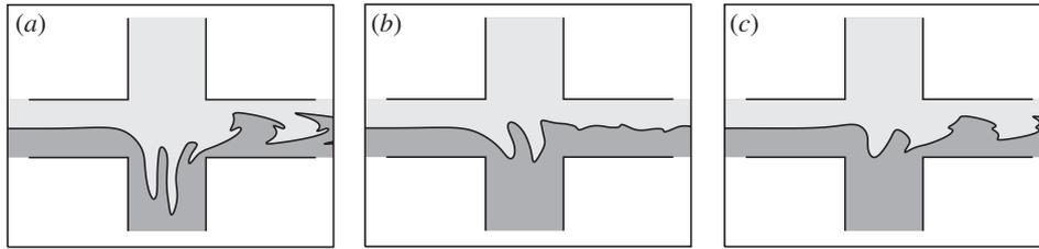
Figure 7. Examples of interface snapshots for different control parameters, showing (a) poor mixing  $\alpha = 5.85$ ,  $\omega = 5.22$ ; (b) strong mixing  $\alpha = 4.85$ ,  $\omega = 5.33$ ; and (c) poor mixing  $\alpha = 3.85$ ,  $\omega = 5.33$ , and thus strong variations in mixing efficiency in narrow regions of the phase diagram of figure 4.
