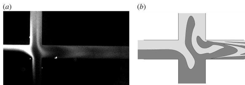
Figure 13. Pattern obtained by (a) experimental and (b) numerical simulations, showing qualitative agreement.
