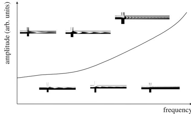
Figure 5. Experimental phase diagram obtained by Lee *et al.* (2001). Horizontal scales are arbitrary, but the order of magnitude of the working frequencies used in the experiment is a few hertz.
