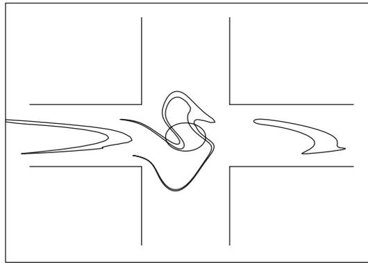
Figure 6. X-mixer with periodic boundary conditions, where snapshots are taken after each full forcing period. The initial round tracer returns strongly deformed to its initial position after three periods, now with a clear horseshoe shape, indicating that the system is truly chaotic.
