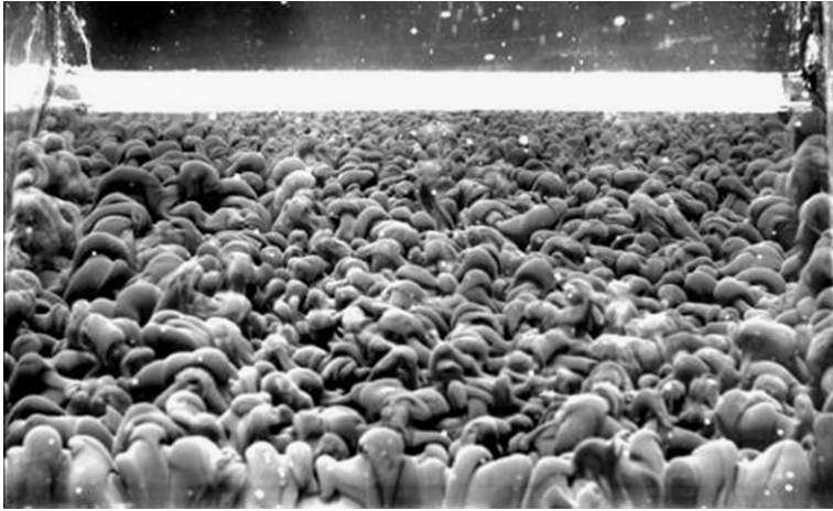
Figure 7. Early three-dimensional development of R–T as the composite barrier (white band near the top of the picture) is withdrawn. (Photograph courtesy of A. G. W. Lawrie, University of Cambridge.)
